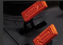
Our hydrostatic drive system (HST) eliminates gear-shifting by safely engaging color-coded forward or reverse pedals. Combining HST with supersmooth joystick control makes front loader work fast and efficient.
