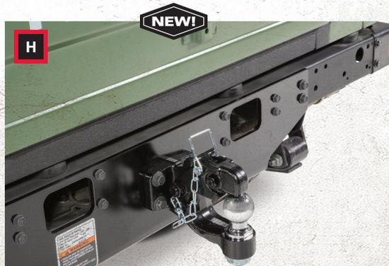
*G. New (optional) lockable pintle hitch with receiver is ideal for heavy-duty off-road towing jobs.*
