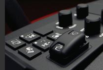
On cab models, the electronic rear hitch controls improve chore efficiency and overall productivity. Easily adjust lift speed, draft, depth, auto-raise on turns, & more.
